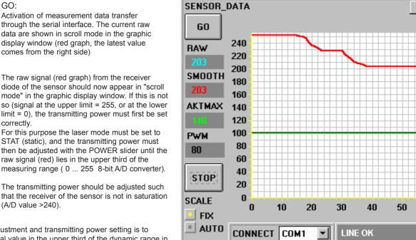
The aim of fine adjustment and transmitting power setting is to achieve a raw signal value in the upper third of the dynamic range in the uncovered situation of the light measuring section ("sensor free").
