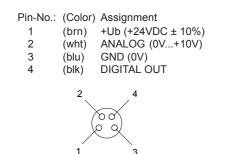
Connecting cable to PLC: cab-M8/4-g-2
