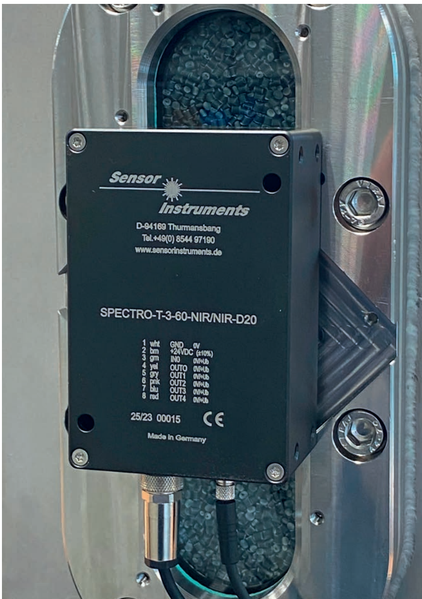
The Spectro-T-3-60-NIR/NIR-D20 NIR inline sensor is mounted on the sight glasses of metering systems and silos. © Sensor Instruments
