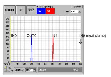
The initiators are mounted in such a way that the position of the two sensors can be freely chosen. Care must be taken to ensure that both sensor 1 and sensor 2 detect every clamp.
