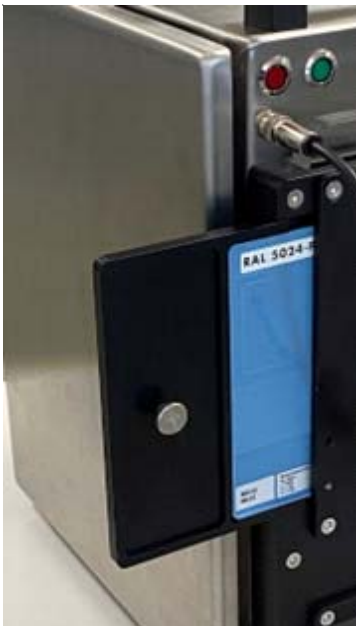
Insertion of an RAL plastic color card
