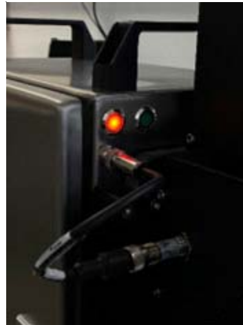
Information via a red LED that the card insertion compartment is empty
