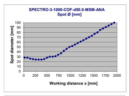
Relative intensity 100% SPECTRO-3-1000-COF-d50.0-MSM-ANA: 100% at a working distance of 860 mm (INTENSITY 3666)
